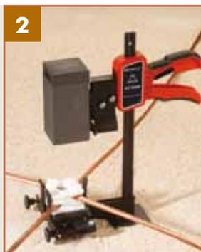
Put the correspondent conductors to be joined, and then another cavity sealer.
