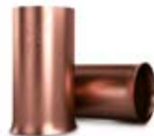
AT-072NCXX: Copper adapter sleeves with variable diameters depending on XX selection. XX indicates the mm 2 of the desired cable. They increase the conductor diameter fitting it in a mould designed for this XX bigger cable. X = 50, 70, 120...
