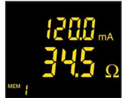
Standard mode: Impedance and leakage current
