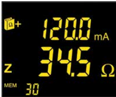
Screen 1: Impedance and leakage current
