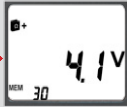
Screen 2: Ground voltage
